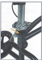
3. Slide locking mechanism into groove on tiller, depress locking handle to secure tiller lock.
